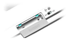
2. Place the 2 AAA-size rechargeable batteries in the battery compartment.
