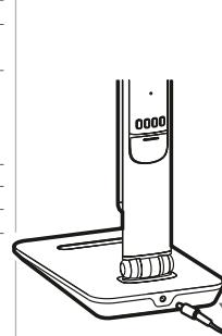
Connect the power adapter in the rear of the lamp arm.
