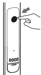
Adjust the brightness of the display by using the touch controls.
