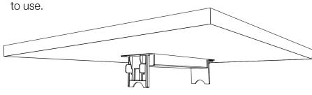
**Note!** To remove the clamps, pull the top part of the clamp② away from the box①. As you pull the top ①, proceed by pulling the clamp downwards until fully removed ②.
