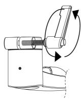
1 Unscrew and position the handle bolt so that the bolt only has contact with one half of the plastic clamp.
