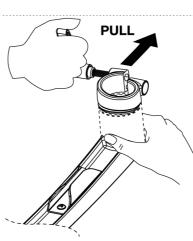
3 As the bottom part of the black plastic surfaces; pull lever outwards until the clamp is completely loose.
