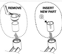
A Remove the black plastic clamp and replace the old bushing with the one provided in the carton box (9). Repeat process with the second arm(8). **Tergo**werken
