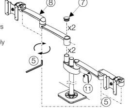
**5** Mount all LCD monitors to the VESA brackets with the provided screws (2) as seen below.
