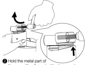
the arm with a firm grip. Use leverage to bend the lever upwards with as much force as possible. The bottom of the clamp will surface as seen in the zoomed-in illustration.
